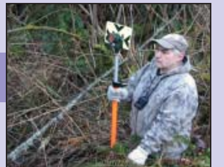
Dwayne Ross Sr. prepares for survey measurement to determine how much road fill separates Clearwater River from its floodplain.
